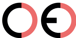
False CE Mark (too far)
